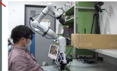
(c) Object selection by gaze from extended visual sensing of the hand-eye RGB-D camera
