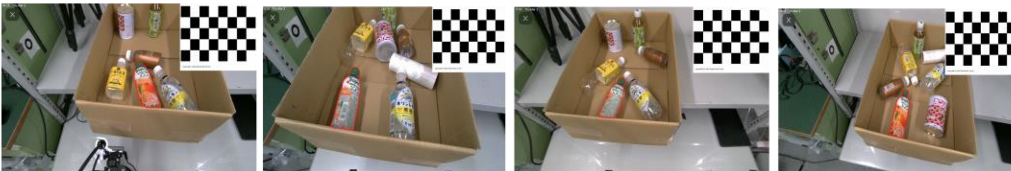
Figure 6. Example images of hand-eye camera shown to the user on the tablet. The chessboard marker in the upper right corner is used to transform the 2D gaze point from the glasses frame to the tablet frame. Red contours indicate the object selection results by the user's gaze.
